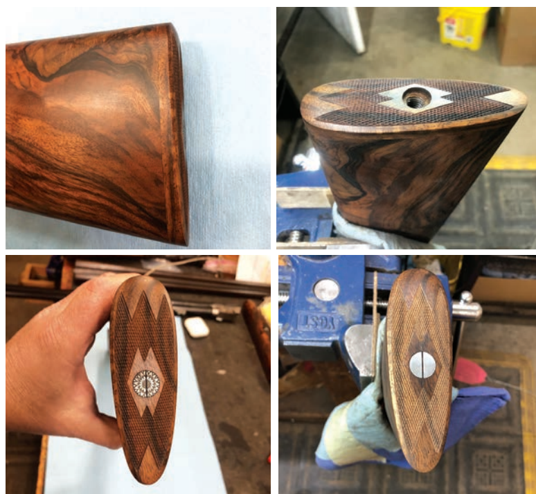
Clockwise from top left: author Del Whitman's "one-screw buttplate" shown from the side, the escutcheon in the hardwood plate to house the "screw," the screw threaded in to cover the drawbolt hole, and the elegant-yet-spare finished treatment.
